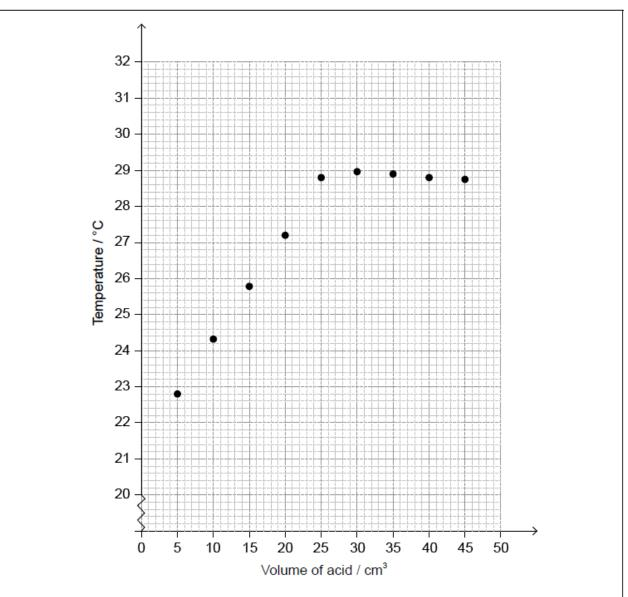
The temperature of the reaction mixture was measured after each acid addition and plotted against the volume of acid.
